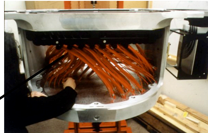
1000 small-core fibers to replace existing (more objects, less sky contamination)
