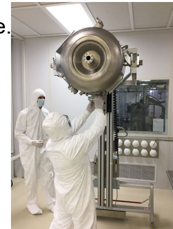
Cavity tooling in the cleanroom minimize the risk of contamination
