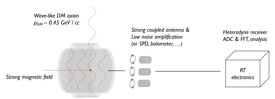
Microwave cavity at axion freq. Conversion power enhanced ( $\sim$  Q)
