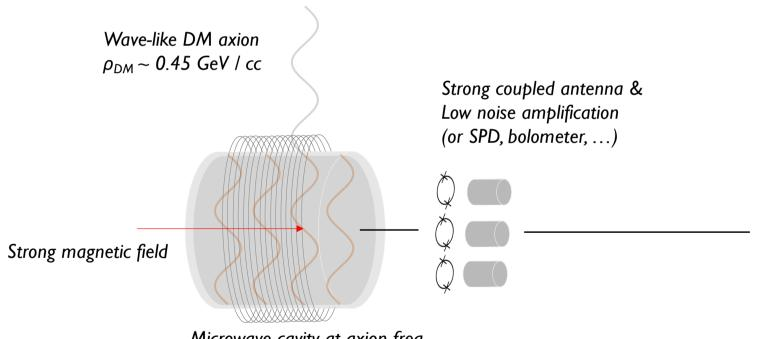
Microwave cavity at axion freq. Conversion power enhanced ( $\sim$  Q)
