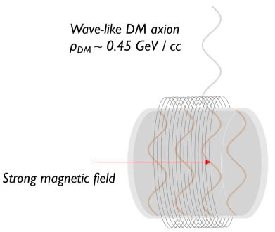
Microwave cavity at axion freq. Conversion power enhanced ( $\sim$  Q)
