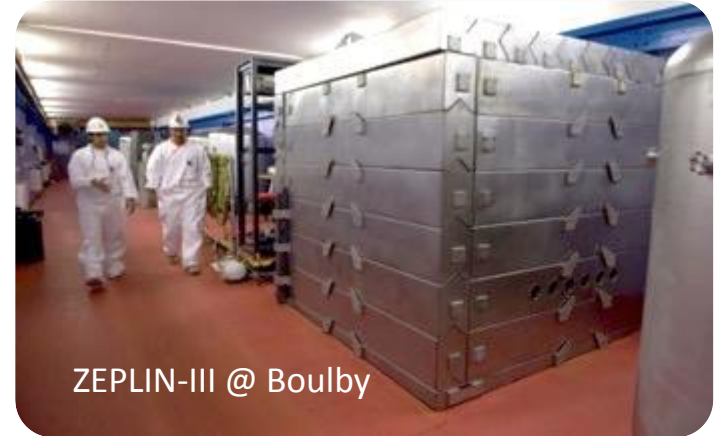
ZEPLIN: The world's first 2-phase Xenon dark matter detector (Finished 2011)
