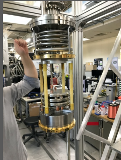
Dilution refrigerator T_{\text{base}} \sim 5.6 \text{ mK} By Leiden
