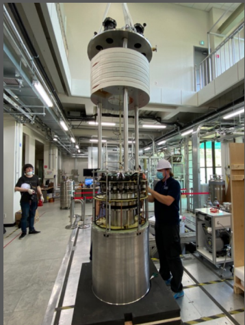
12 Tesla SC magnet 320mm bore diameter By Oxford. Inc
